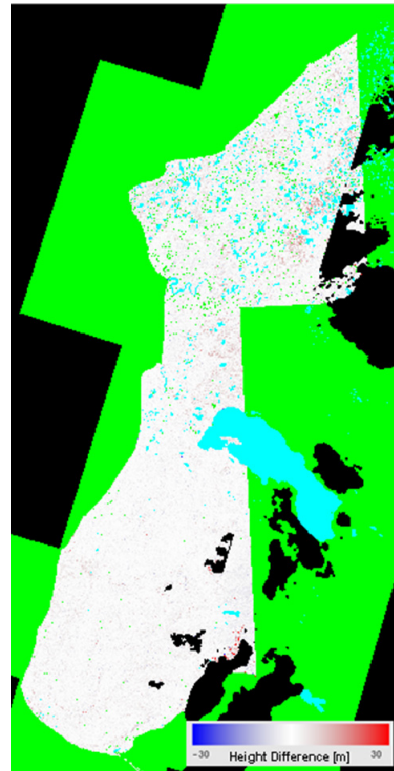
Figure 3. Height difference between generated PRISM DSM and airborne Lidar (black and sky blue: masked out areas)
